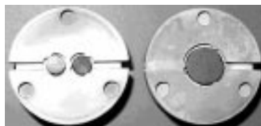
Fig. 4 Photographs of specimen holders for 5 mm diameter (left) and 10 mm diameter (right), respectively
